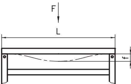
$$f [\text{mm}] = \frac{0.0074 \times F [\text{N}] \times L^3 [\text{m}]}{I [\text{cm}^4]}$$
