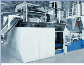
Machine base frame and housing
