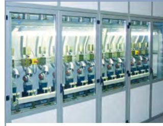
Protective cabinet and noise protection
