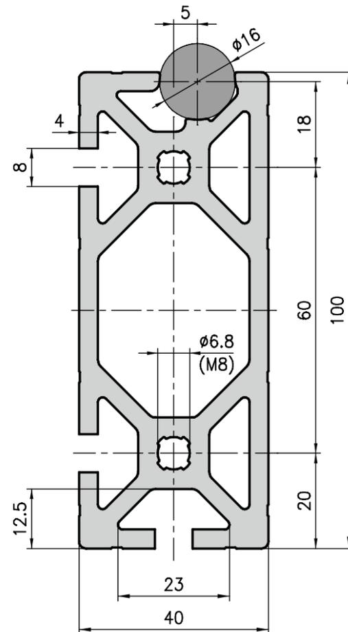
the front face in the holes Ø 6.8 with a M8 thread.
