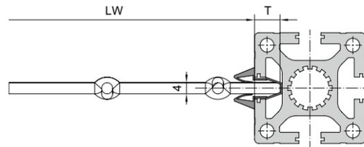
Application with grid extrusion C39-70
