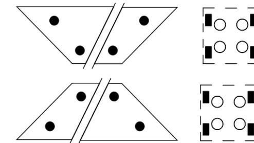
Mitre cut + PVS® hole(s) acc. to customer drawing
