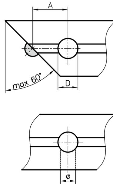
That drill, allows a connection for a parallel connector at any position at the extrusion.
