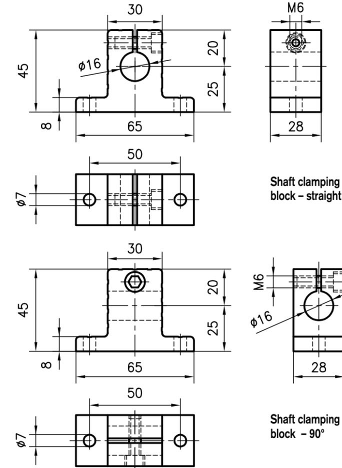
Shaft clamping block - straight
