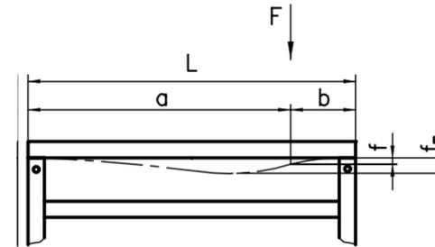
$$f [\text{mm}] = \frac{0.476 \times F [\text{N}] \times a^3 [\text{m}] \times b^3 [\text{m}]}{I [\text{cm}^4] \times L^3 [\text{m}]}$$
