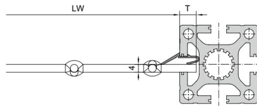
Application with wedge extrusion C39-45
