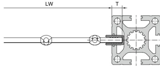
Application with U-Clamping extrusion B19-6
