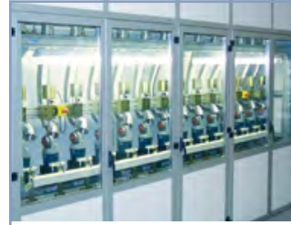
Protective cabinet and noise protection
